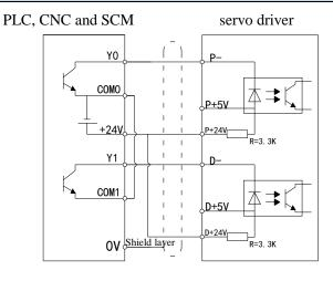
When the upper device adopts collector open circuit output, use this connection method, please pay attention to suspending P+ 5V and D+ 5V.
