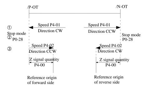
Sequential diagram of finding reference origin on forward side:
