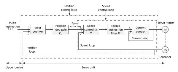
Position control loop diagram (shut down the model loop)
