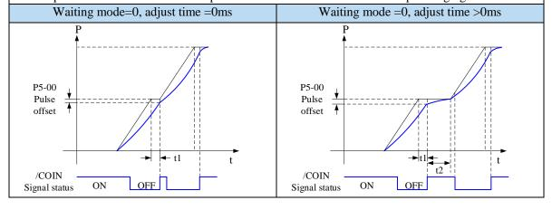
After the drive output 1-segment position command, it will wait for the completion of motor positioning, and then start the next position command at once. T1 is positioning time, which means the time from pulse output complete to the output of positioning completion signal.
