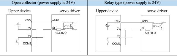
Note: SI10 terminal is high-speed input port, and SI1-SI9 are low-speed input ports.
