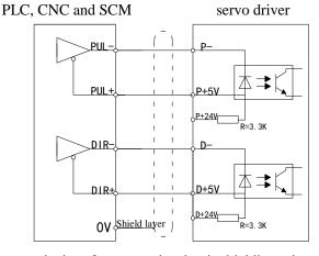
When the upper device uses 5V differential signal output, the graphic connection method is adopted, please pay attention to suspending P+ 24V and D+ 24V.
