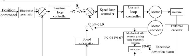
When the full closed-loop is opened, the external grating ruler position feedback is used; when the full closed-loop speed feedback is opened, the external grating ruler speed feedback is used. When the full closed-loop mode is on, the control mode can be switched (P0-01 and P0-02).
