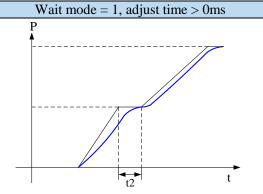
After the drive output 1-segment position command, it will not wait for the completion of motor positioning, but pass the adjust time, and then start the next position command. T2 is adjust time. Refer to parameter P4-11.
