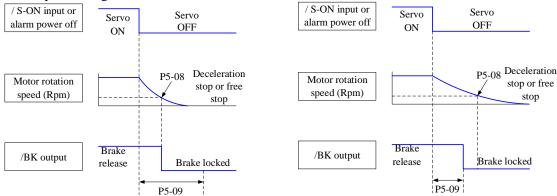
Since the brake of the servo motor is designed for position holding, it must be enabled at the right time when the motor stops. While observing the action of the machine, adjust the user parameters.
