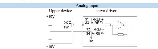
Note: Analog Pin31 (External Torque Analog Differential Input+), 32 (External Torque Analog Differential Input+), 33 (External Speed Analog Differential Input+), 34 (External Speed Analog Differential Input+) are soldered out of the CN0 port as detailed in chapter 3.1.3.1.
