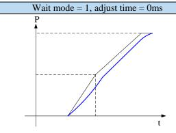
After the drive output 1-segment position command, it will not wait for the completion of motor positioning, and start the next position command at once.
